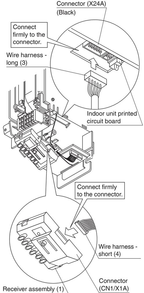
After making these connection, clamp the wire harness - long (3) and the wire harness - short (4) using the included clamp (7).
