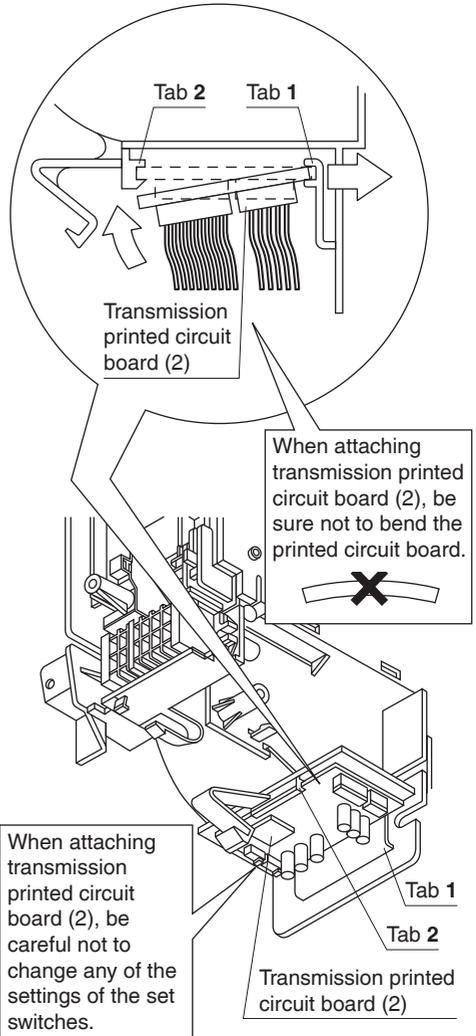
3. Attach the included receiver assembly (1) to the 2 tabs on the indoor unit, as per the figure.
