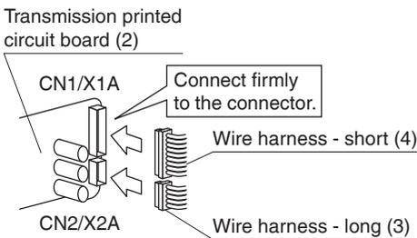
2. Following the figure, insert transmission printed circuit board (2) into tab 1, then insert into tab 2 while pushing tab 1 in the direction of the arrow.
